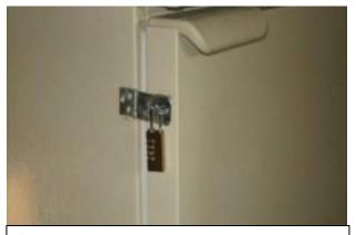
Super glue was used to apply the above padlock to a lower freezer door. No drill was used; so the risk of hitting Freon coils was prevented.
